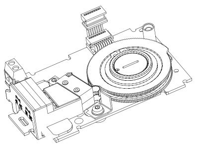
Figure 5-6 Mechanical limit switch module
