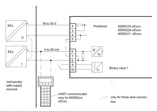
Figure 6-12 Three/four-wire connection, Ex i
