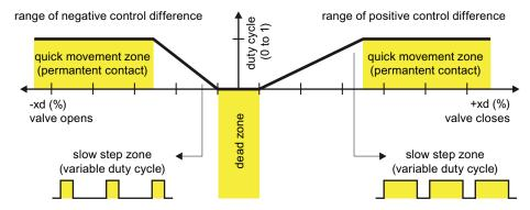
Figure 3-15 Functional principle of five-point controller
