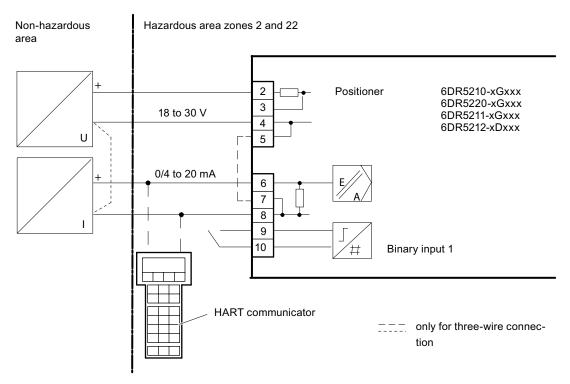
Figure 6-21 Three/four-wire connection, Ex n
