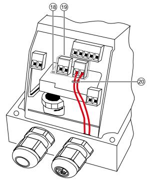
Figure 6-9 Connecting the cables
