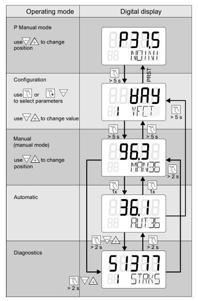
Figure 7-3 Switching between the operating modes
