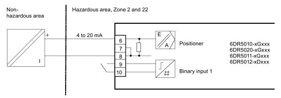
Figure 6-19 Two-wire connection, Ex n
