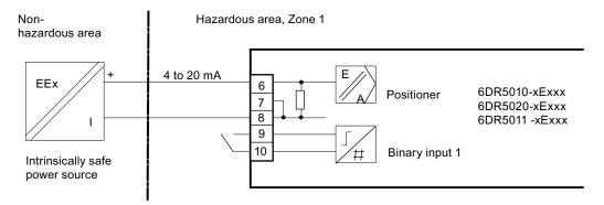
Figure 6-10 Two-wire connection, Ex i
