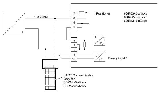
Figure 6-3 Two-wire connection for 2-, 3-, 4-wire version
