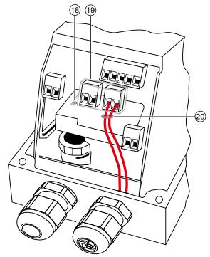
Figure 6-26 Connecting the cables
