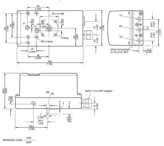
Figure 14-1 Dimensions of plastic enclosure version
