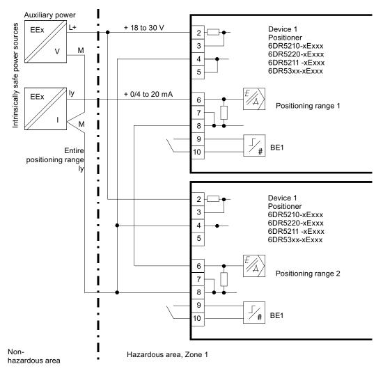
Figure 6-13 Series connection of 2 positioners, e.g. split range (auxiliary power wired separately), EEx i
