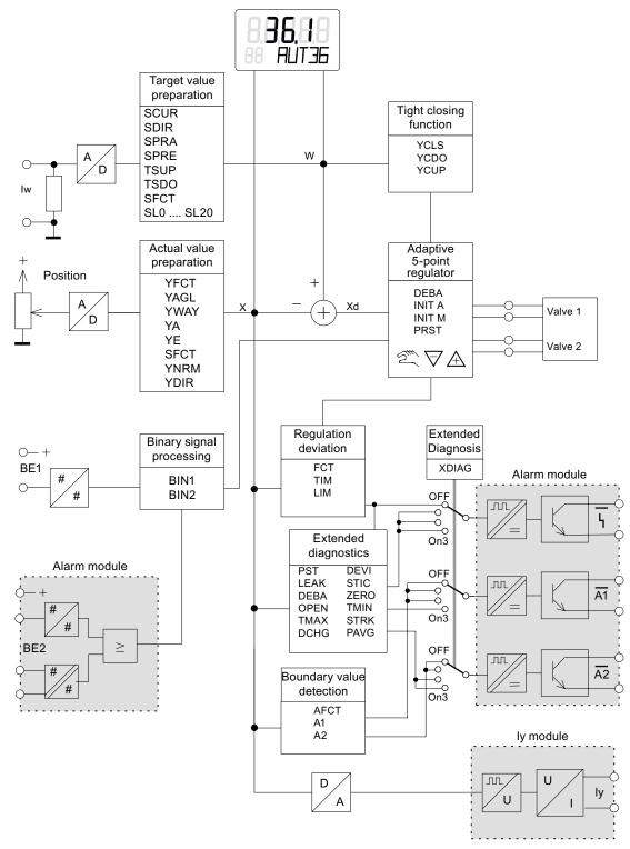
Figure 10-1 Configuration block schematic
