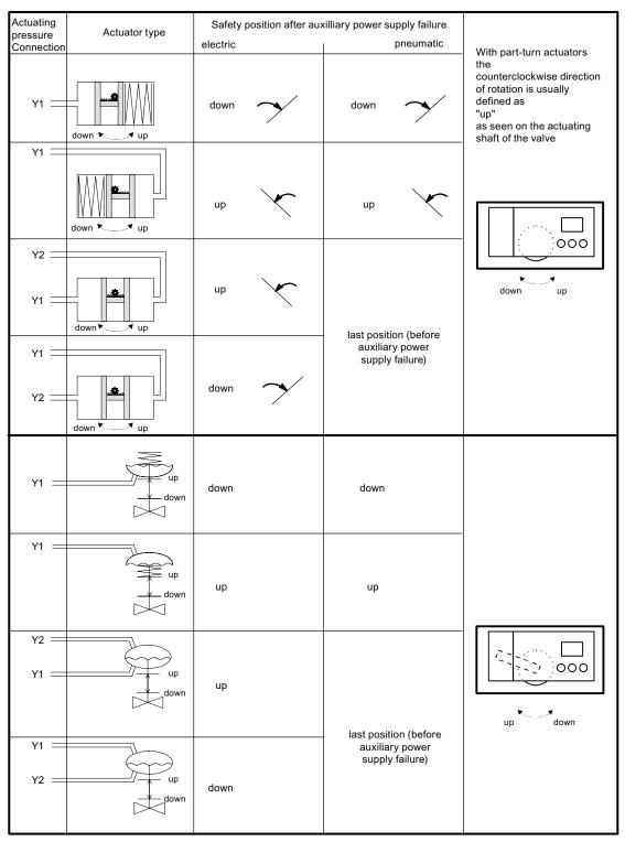
Figure 3-12 Regulating action of pneumatic connection
