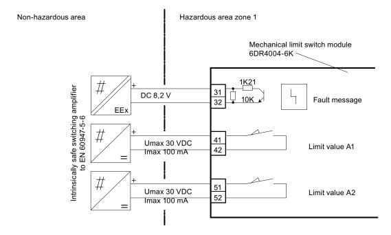
Figure 6-17 Mechanical limit switch module 6DR4004-6K, Ex i
