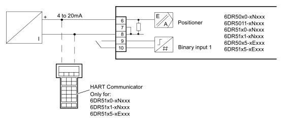
Figure 6-2 Two-wire connection
