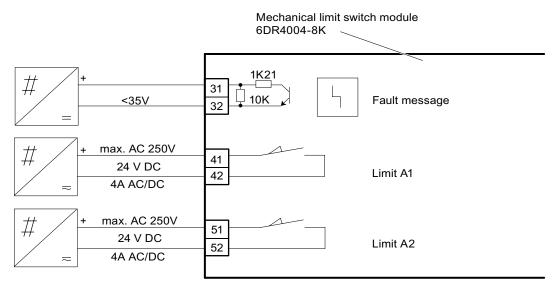
Figure 6-8 Mechanical limit switch module 6DR4004-8K, not Ex
