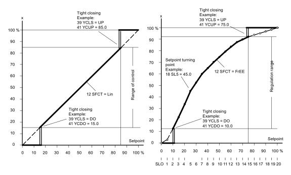
Setpoint characteristic curves, standardization of manipulated variables, and tight closing function
