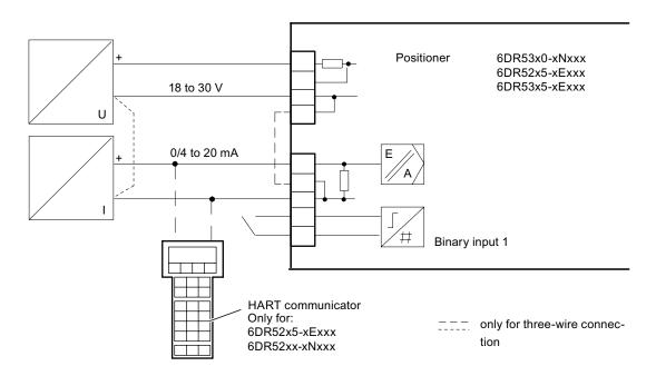
Figure 6-4 Three/four-wire connection
