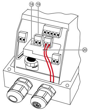
Figure 6-18 Connecting the cables
