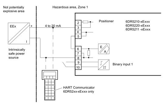
Figure 6-11 Two-wire connection, Ex i
