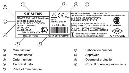
Figure 3-5 Structure of the nameplate, example
