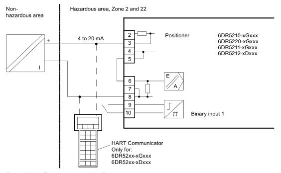
Figure 6-20 Two-wire connection, Ex n
