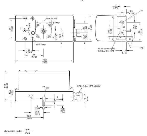
Figure 14-3 Dimensions of metal housing version
