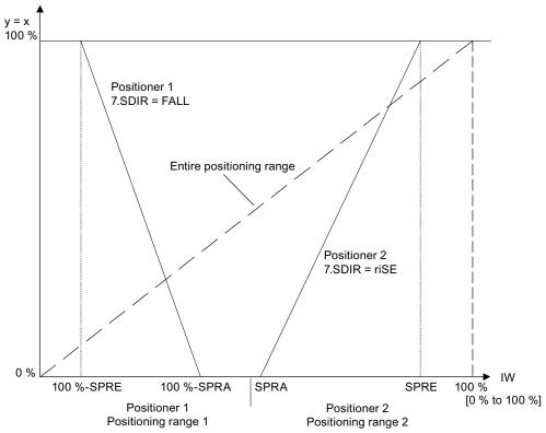
Figure 10-2 Example: Split range operation with two positioners
