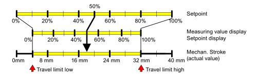
Figure 10-5 Example: YNRM = FLOW with YA = 10 % and YE = 80 %
