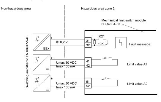
Figure 6-25 Mechanical limit switch module 6DR4004-6K, Ex n
