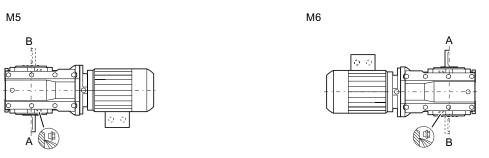
Figure 10-2 Mounting position for bevel gearbox B foot-mounted design, size 29
