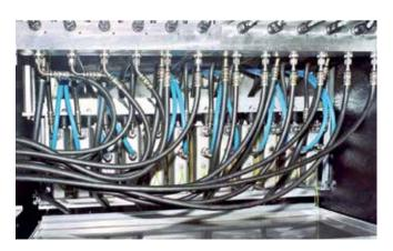
12 SITRANS F C Coriolis flowmeters improve the performance of test benches for the automotive industry. The rugged construction and precisely trimmed pipe loops render the sensor insensitive to process noise, vibrations and water hammers. The resulting stable zero point ensures a wide dynamic range.
