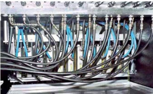
12 SITRANS F C Coriolis flowmeters improve the performance of test benches for the automotive industry. The rugged construction and precisely trimmed pipe loops render the sensor insensitive to process noise, vibrations and water hammers. The resulting stable zero point ensures a wide dynamic range.
